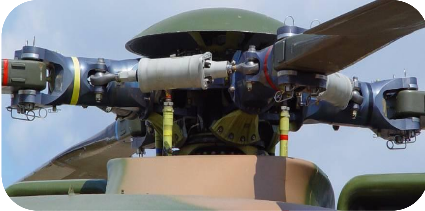
Main rotor lead lag dampers and pitch control rod ends
