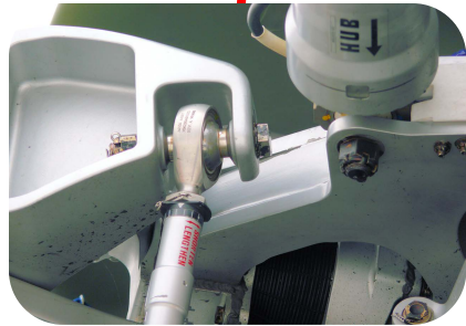
Main rotor lead lag dampers and pitch control rod ends
