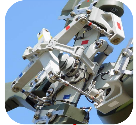
Tail rotor pitch control rod ends and feathering bearings
