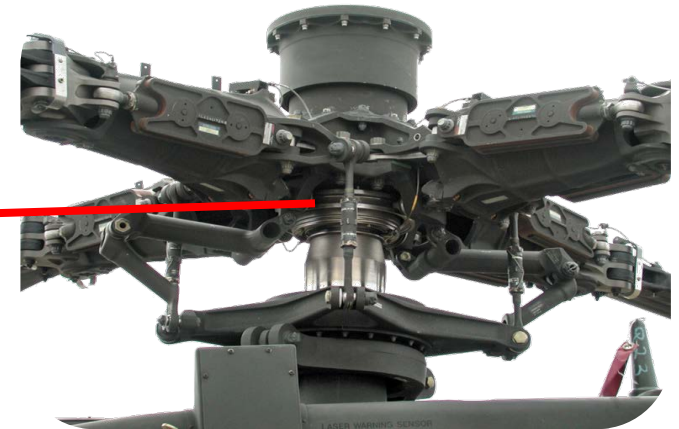
Main rotor: -Pitch control rod ends (XLNT)
