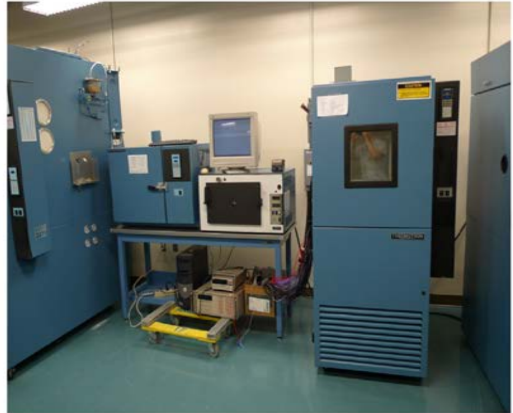
Thermal Cycling Test -40 to 125° C
