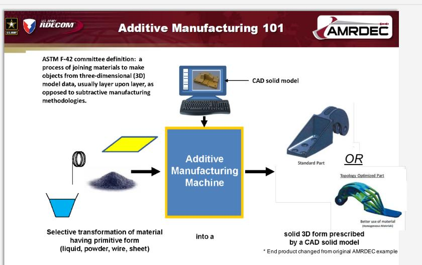
AM enables a new design realm in which geometric complexity is not a constraint, and material can be located where you need it, and not where you don't need it.
