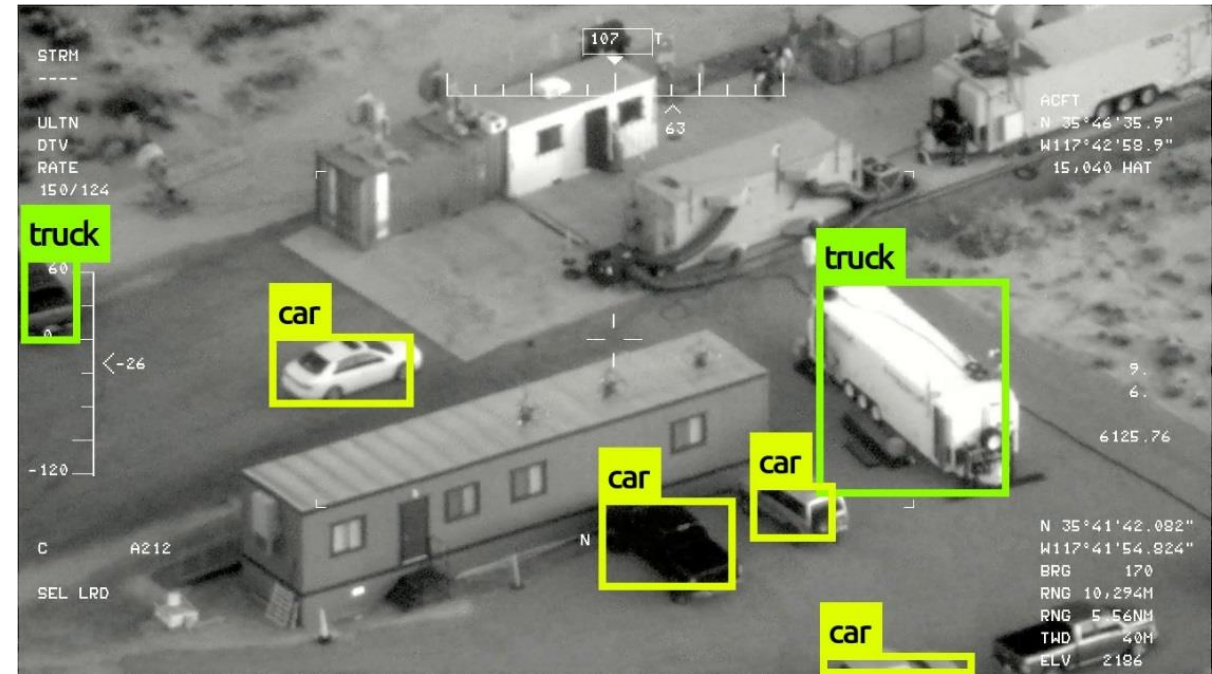
UAV footage with cars and trucks recognized and highlighted.
