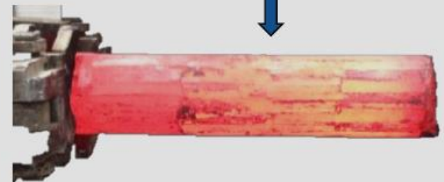
Intermediate press forged to 7" Rd
