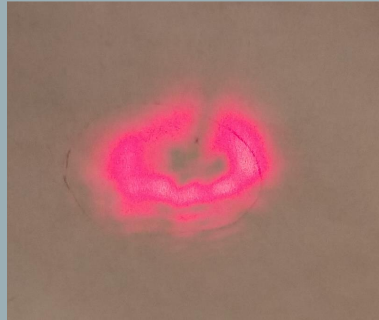
Intensity pattern from an OAM beam
