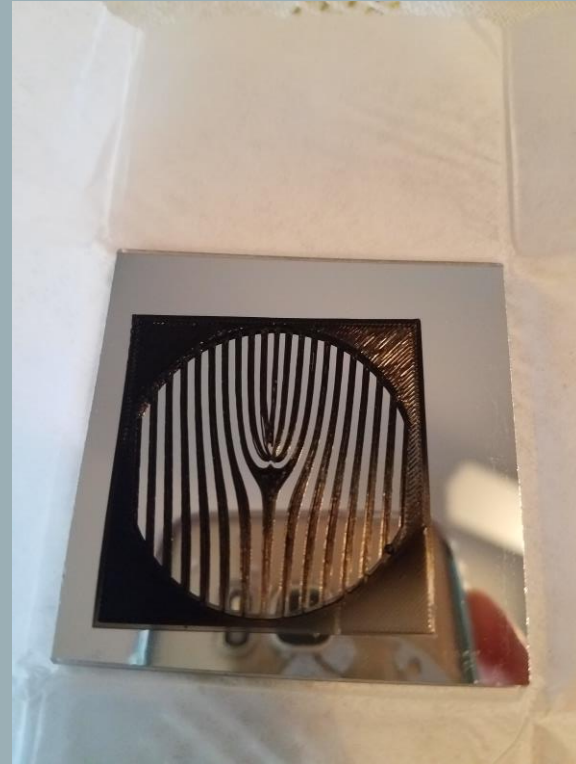
Higher l value ( l = 6 ) printed on a mirror
