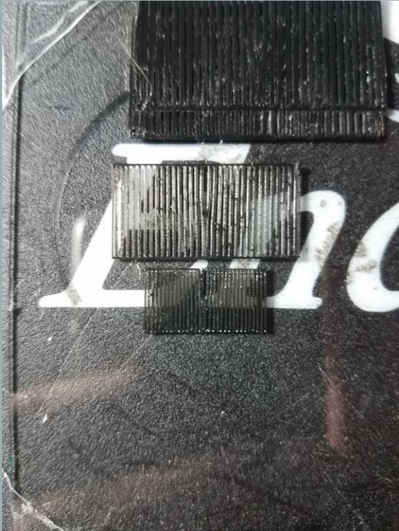
Original size compared to the 0.2mm nozzle size
