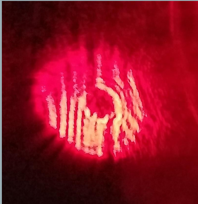
OAM without m = 2, 3, \dots being blocked by slit
