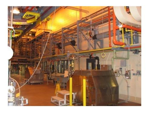
Two homogenizers designed to operate at 8000 psi to break open cells.
